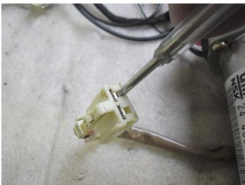
Use a small screwdriver to push back the clip inside the housing. Pull the connector from the housing at the same time.
