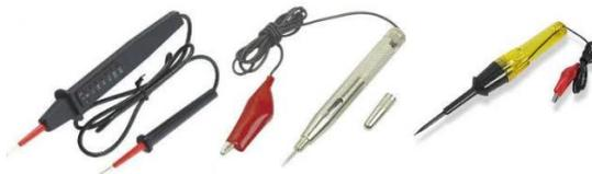
If you switch on the ignition and turn the potentiometer (rheostat) anti-clockwise (to the left) for maximum support, now you can measure between the car's ground/earth and the controller's blue wire. There should be a flashing light visible. If you turn the potentiometer to the right, the flashing speed will increase.
