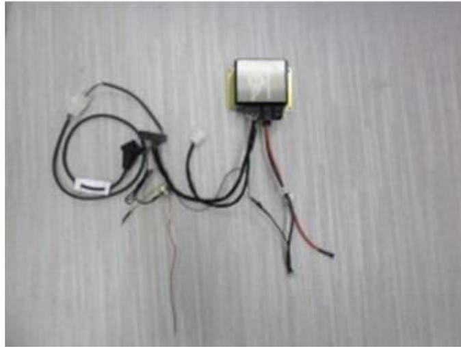
1. Connect the wire harness with the power steering ECU.
